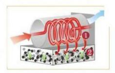
Two dust chambers keep dust from entering the cyclonic ch—amber and ensure a better wo—rking condition of the cyclone.
